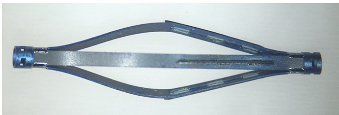
Figure 2: Nitinol laser cut hypotubes—Used to deliver therapy
